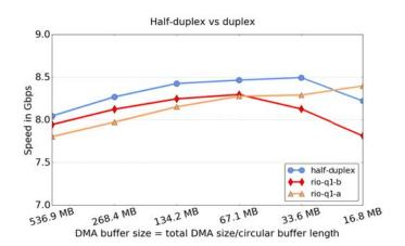
Figure 5. ROOT - half-duplex vs duplex.
